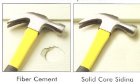
Hammer Impact Test
